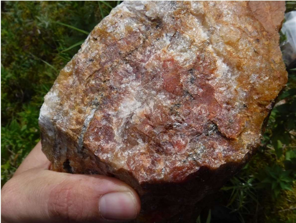
Figure 3: Hematized quartz vein with abundant pyrite and local chalcopyrite, trench area 2.
