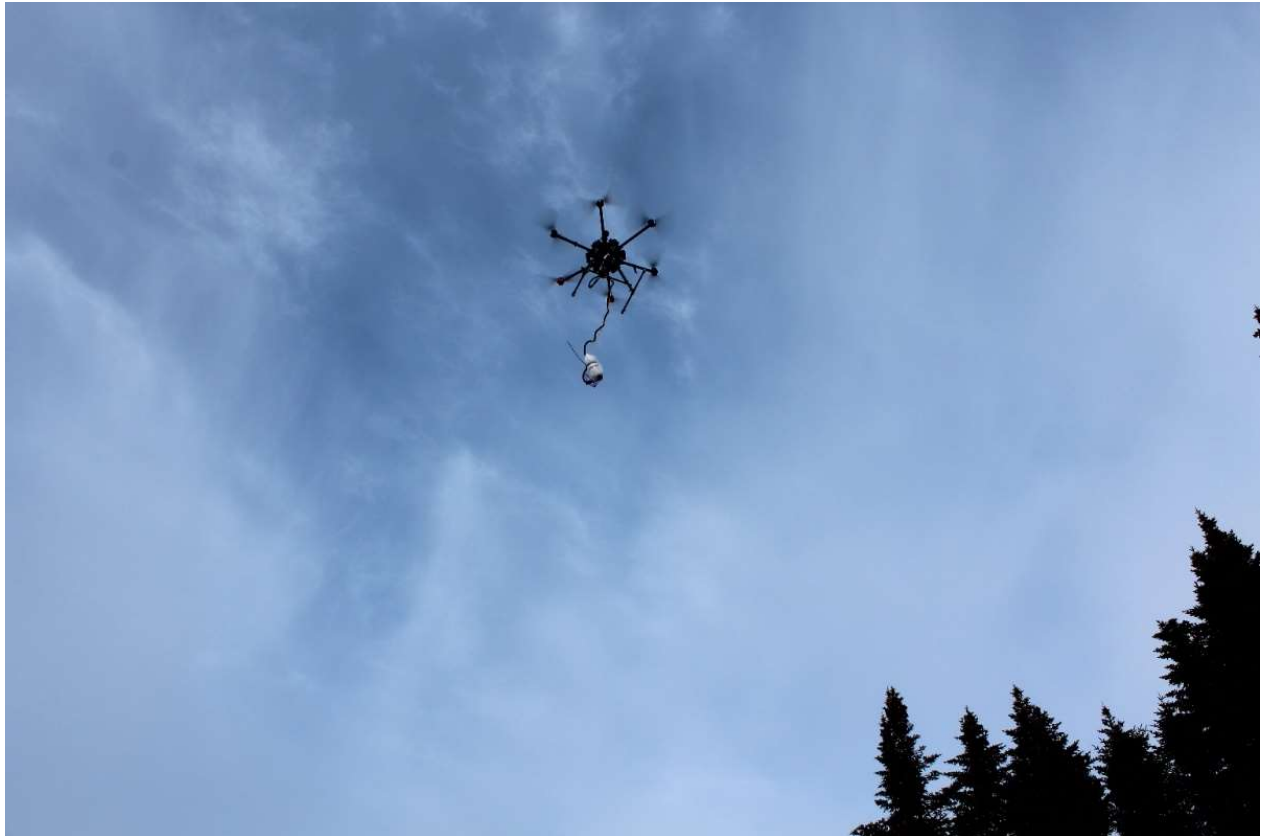
Figure 4: MWH Drone and Magnetometer.
