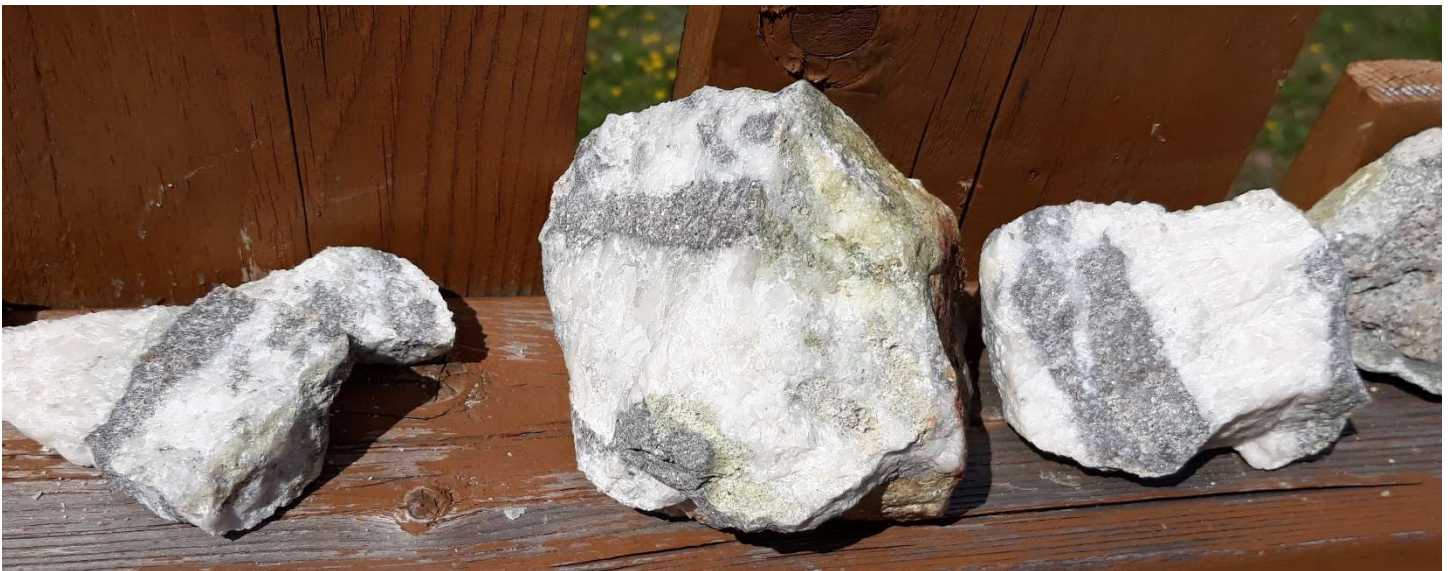
Figure 2: Bands of fine-grained Pyrite and Arsenopyrite in quartz.
