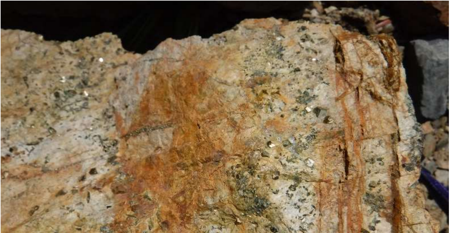
Figure 1: Au bearing Pyrite, Arsenopyrite host rock, Trench #4, Middle River Gold
