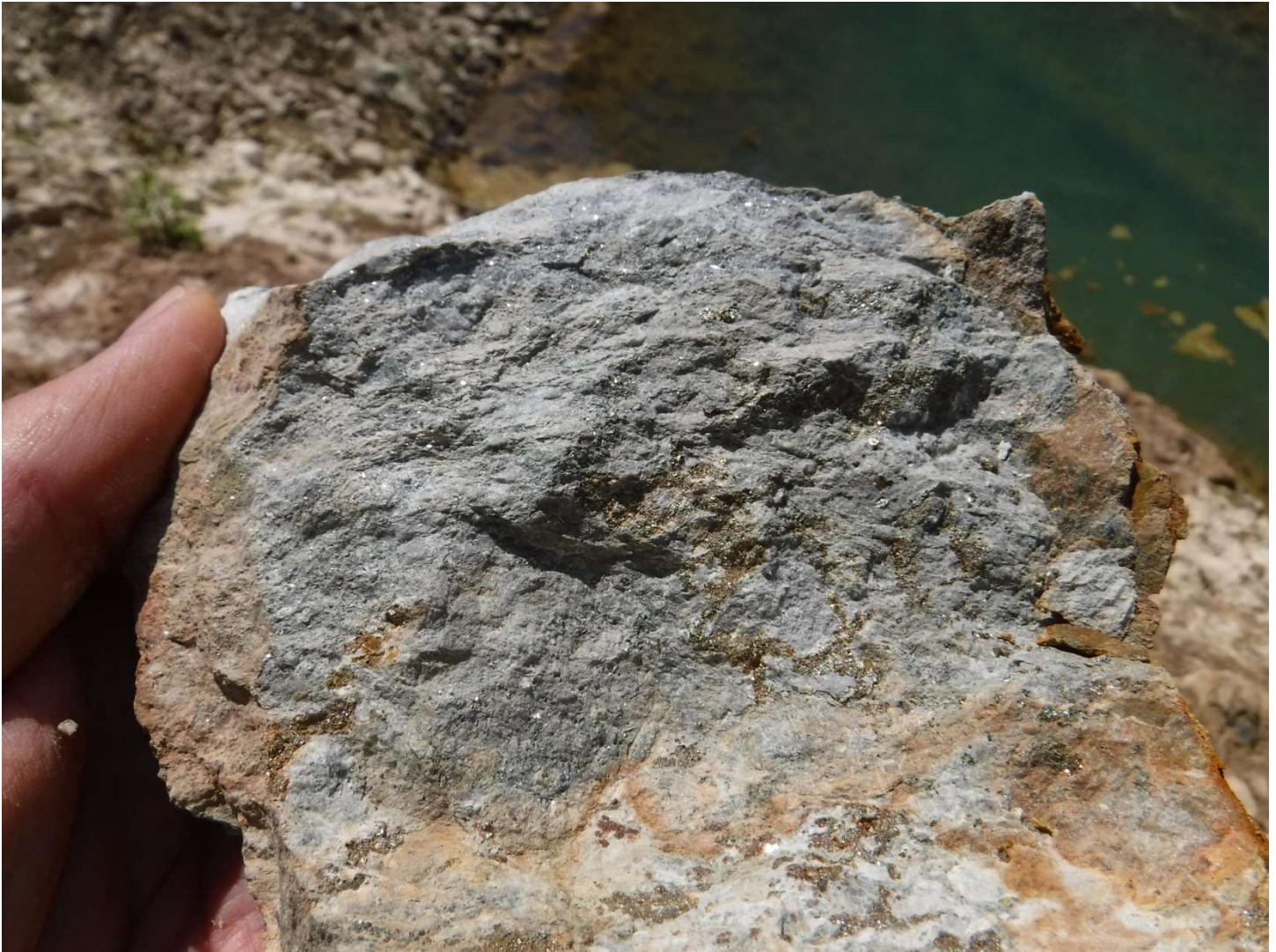
Figure 3: Fine grained Pyrite and Arsenopyrite, Trench #4, Middle River Gold
