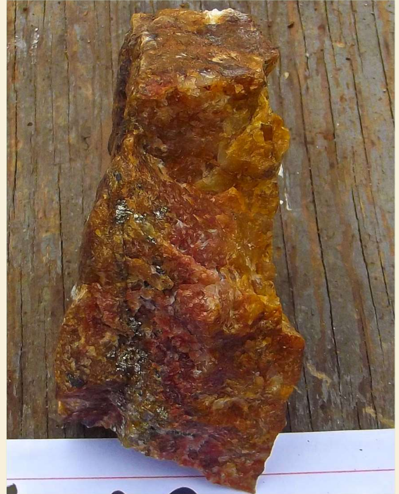
Sample 20CG0003. Oxidized quartz vein with abundant pyrite 1.625 g/t Au, 34.6 g/t Ag, 30 ppm Tungsten
