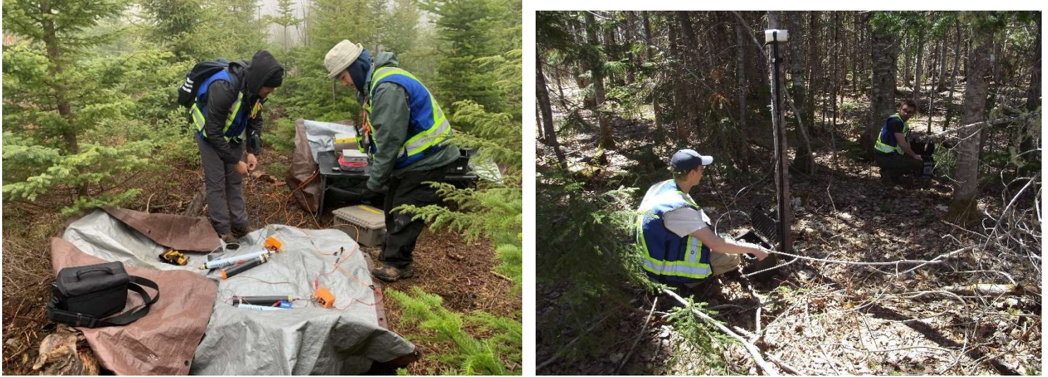
Figure 3: Ground Base Station, Transmitter, TDEM Survey
